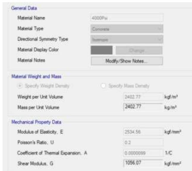
The screenshot displays the material input dialog box in Etabs software, organized into three sections:
