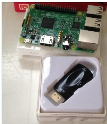
FIGURA 4. 2 : Tarjeta interna Raspberry Pi 3 MB
